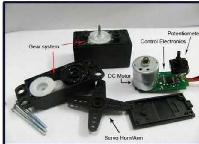
Fig 4 Dc Servo motor [5]
