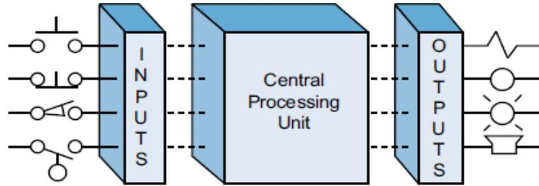
Fig 1 Programmable controller block diagram [3].
