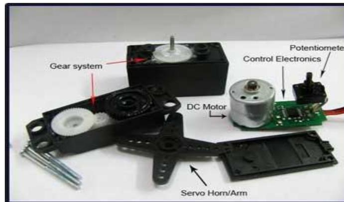
Fig 4 Dc Servo motor [8]
