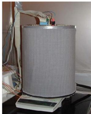
Figure 7. A sweating cylinder for measuring heat and moisture transmission through clothing materials
