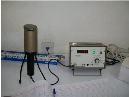
Figure.(1) shows 125I Gamma Counting single channel
