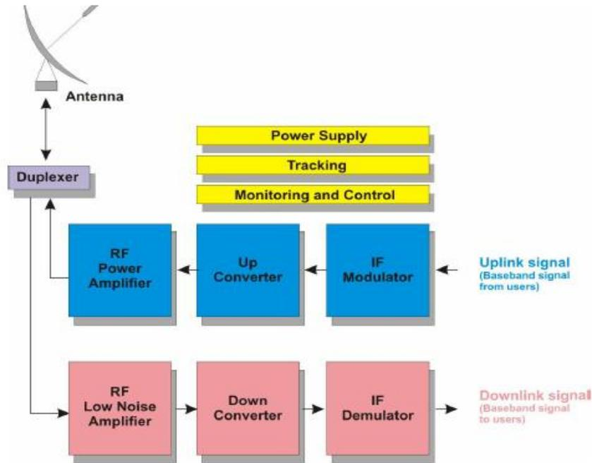
Figure 1: Satellite System Components
