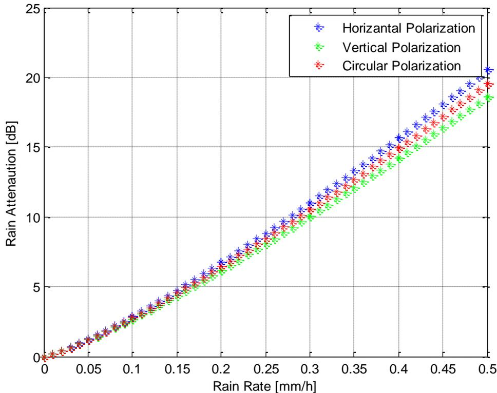
**Figure 3: Rain Attenuation and its Rate**
