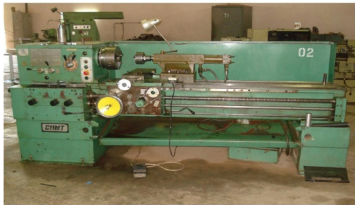
Figure 1. The lathe machine modified into a friction welding machine
