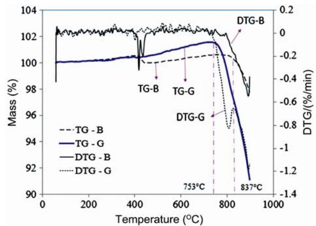
Fig. 3—TG and DTG curves for nonwoven basalt and glass fabrics characteristic parameters of thermal decomposition of nonwoven basalt and glass fabrics obtained from TG curves are shown in Table 5.
