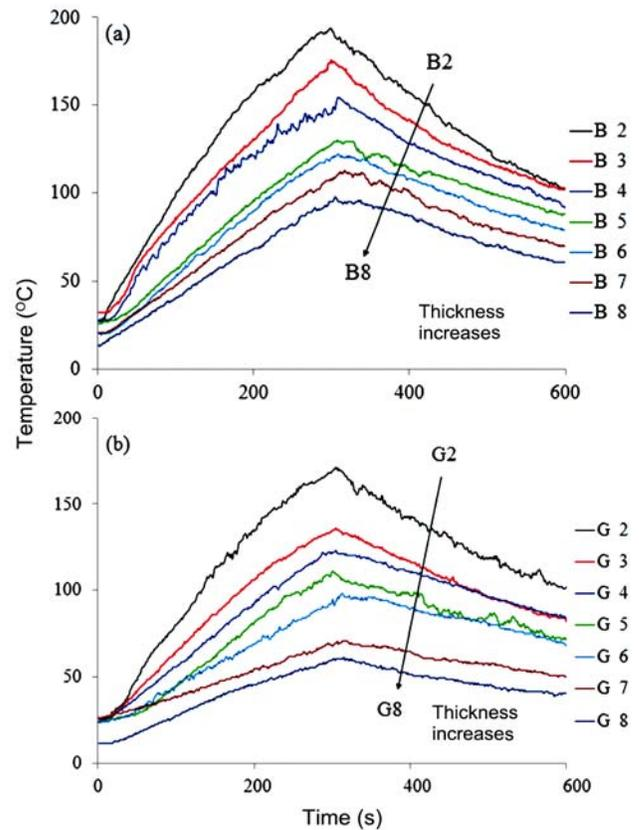
Fig. 4—TPP test for nonwoven (a) basalt and (b) glass fabrics
