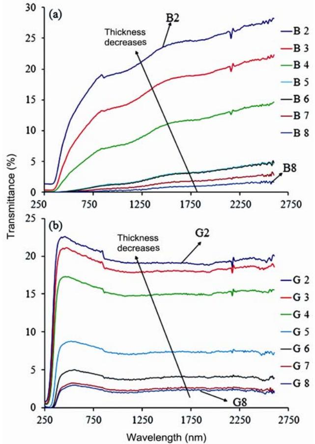
Fig. 2—Spectral transmittance for nonwoven (a) basalt and (b) glass fabrics
