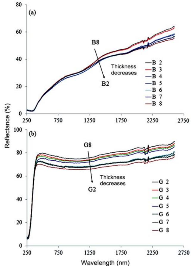
Fig. 1—Spectral reflectance for nonwoven (a) basalt and (b) glass fabrics
