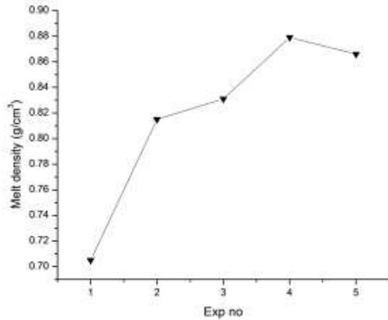
**Figure4. The Melt density of PP/LLDPE and composition**
