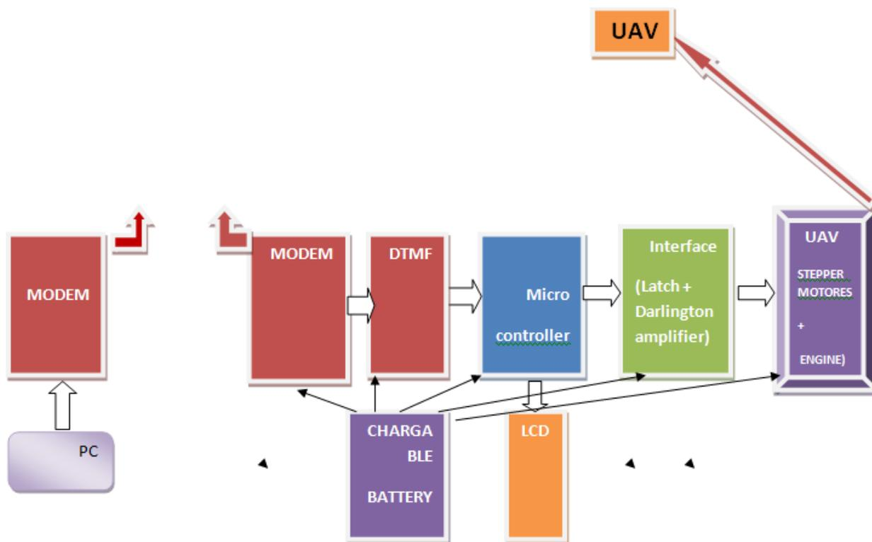
Figure (1) block diagram of the UAV remote control system
