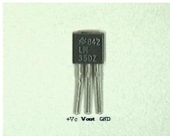
Figure (2) LM35 temperature sensor
