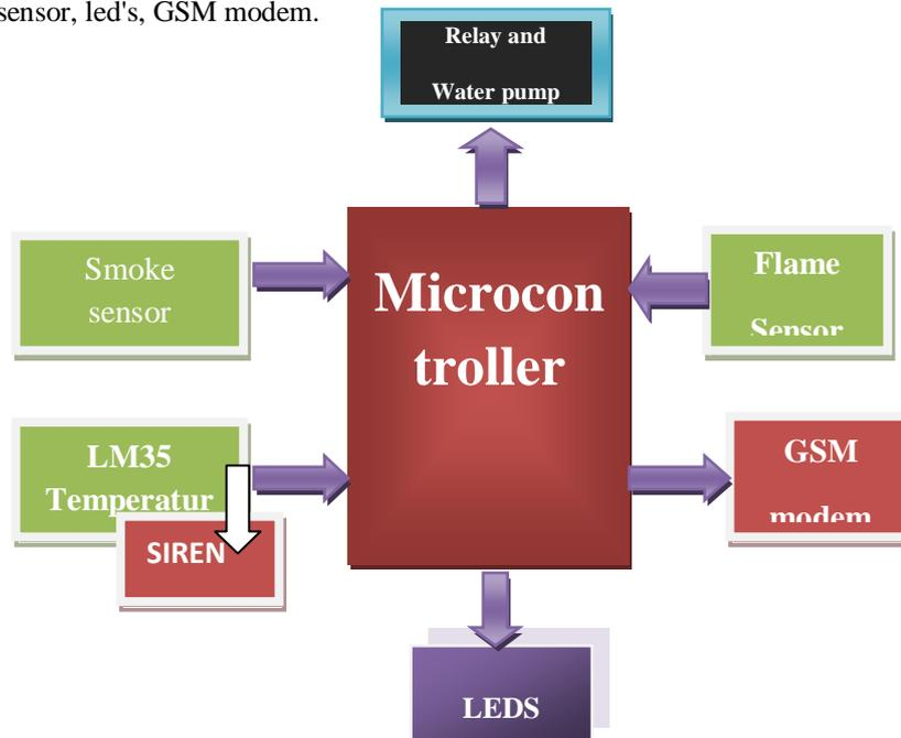
Figure (1) Block diagram of the wireless fire fighting system
