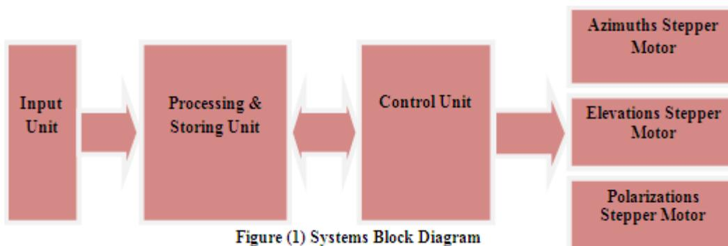
Figure (1) Systems Block Diagram
