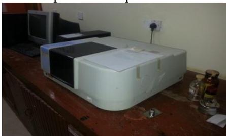
Figure 5: Shimadzu IR Spectrophotometer device
