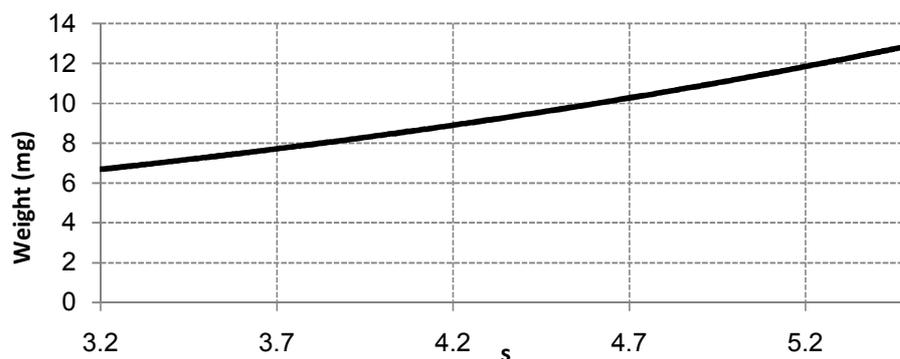
Fig. 13: Weight – breaking load for darkly pigmented wool bleached by reducing followed by oxidizing method
