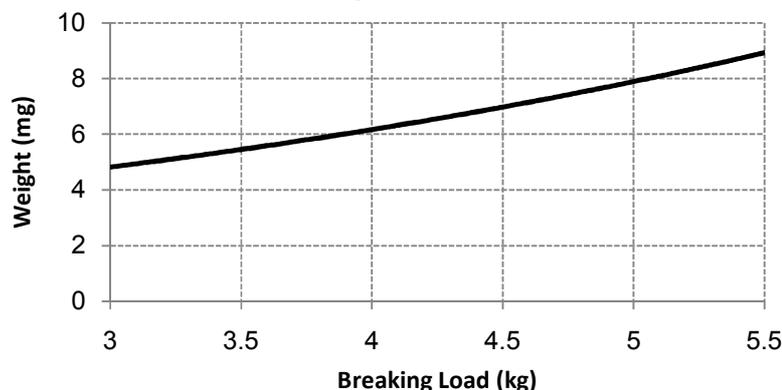
Fig. 12: Weight – breaking load for darkly pigmented wool bleached by oxidizing method
