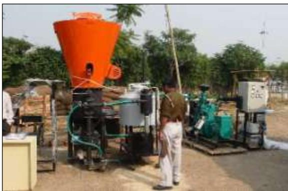
Fig. 6. An Indian-made 10 kW-e gasifier, designed to run on dry woody biomass (i.e., chunks of dried *jatropha* prunings)
