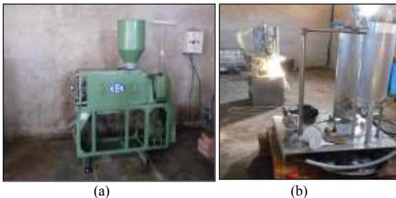
Fig. 5. (a) Small *jatropha* oil extraction machinery being used in Zambia (b) Crude-*jatropha*-oil filtering systems in use in Zambia to produce oil clean enough for fuelling modified diesel motors (in pumps and generators and vehicles)
