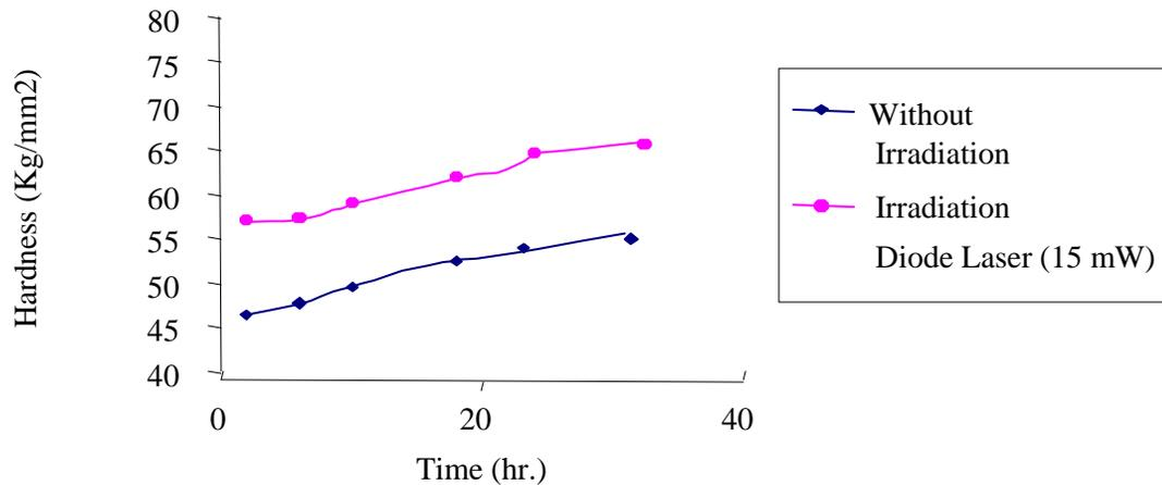
Fig. 1 The hardness of samples without irradiation and of that irradiated by diode laser after different time intervals.
