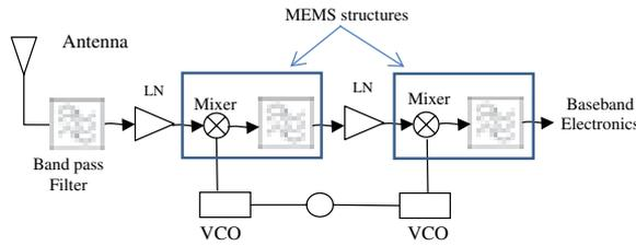
**Fig. 1.** Simple block diagram for wireless receiver, replacing the shaded area with a micromechanical device (Nguyen and Wong 2004).
