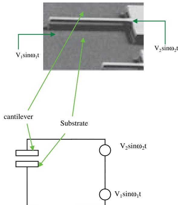
Fig. 3. Circuit diagram of the signal multiplication on electrostatic cantilever.
