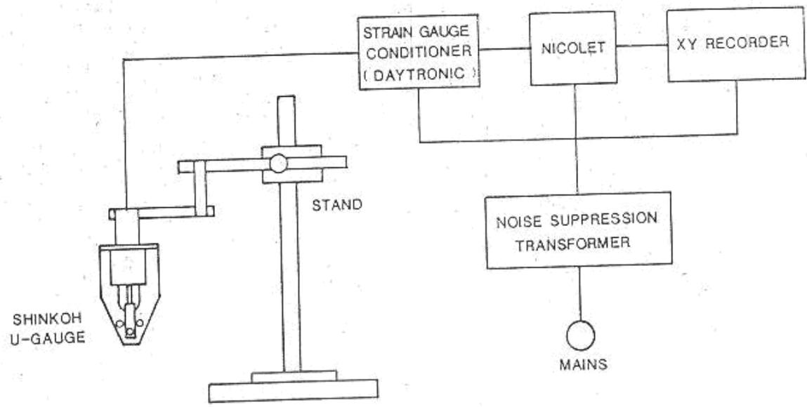
**Fig. (1): Experimental Arrangement for Measuring the yarn Tension**
