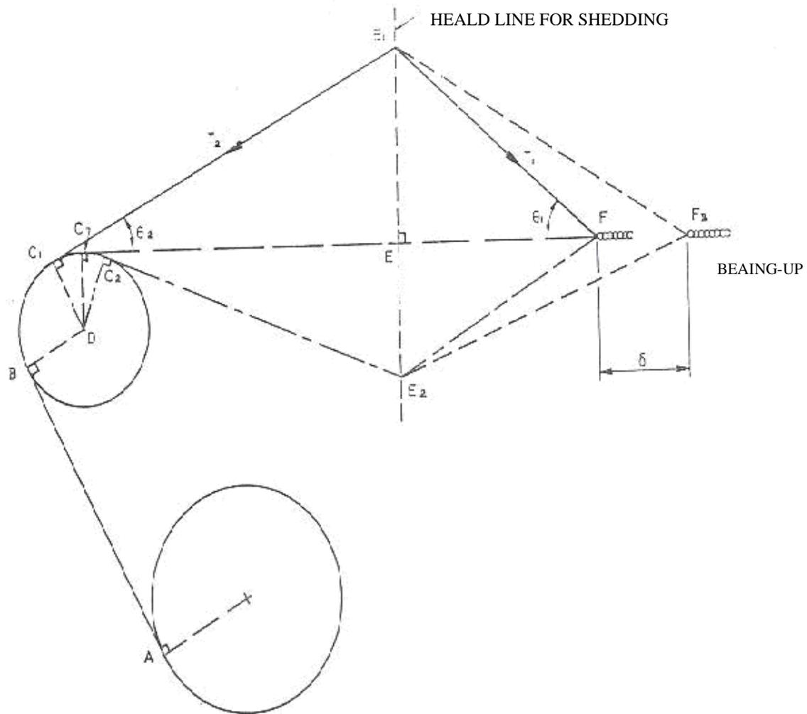
**Fig. (2): Geometry of warp yarns for two consecutive shafts**
