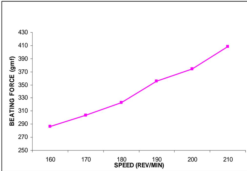
**Fig. (3): The Beating Force as Function of Loom Speeds**
