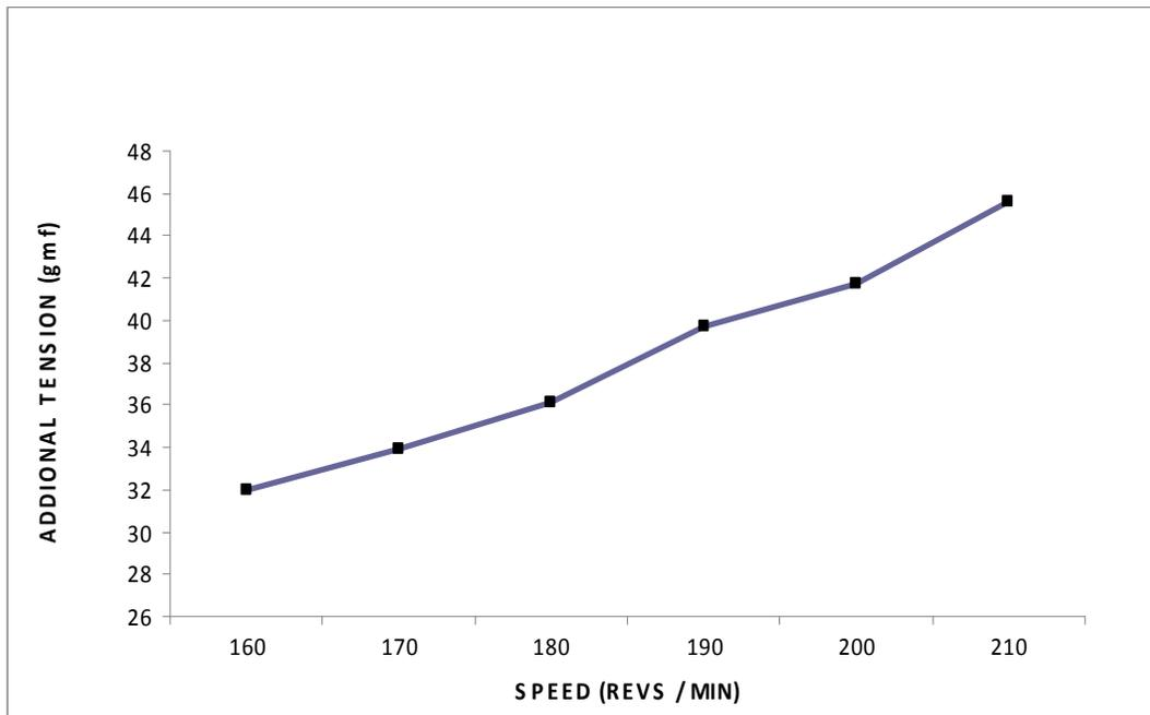
**Fig. (4): The Additional Yarn Tension ( $\Delta T$ )<sub>y</sub> Caused By the Beating Action at Different Loom Speeds**
