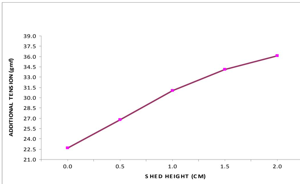
**Fig. (6): The Additional Yarn Tension Caused By the Beating Action at Different Shed Heights**
