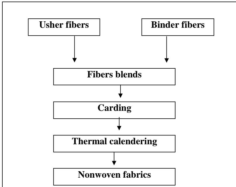
**Figure (2): nonwoven fabric made of usher - Ester fibers
