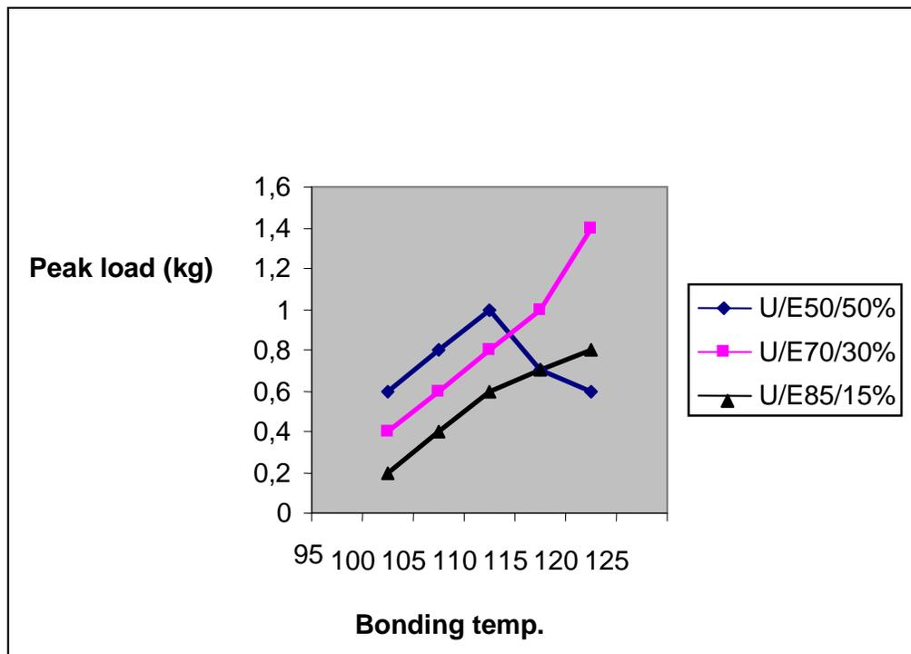
Fig. (3) : effect of bonding temperature on peak load
