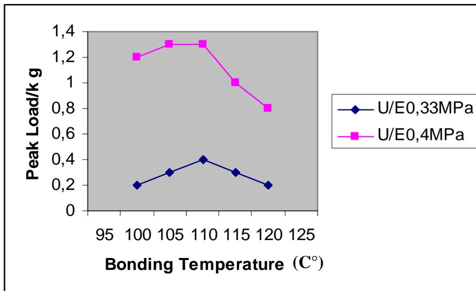
**Fig. (5): Relations between Bonding temperature and peak loads for 30/70 Usher/ ESTER**
