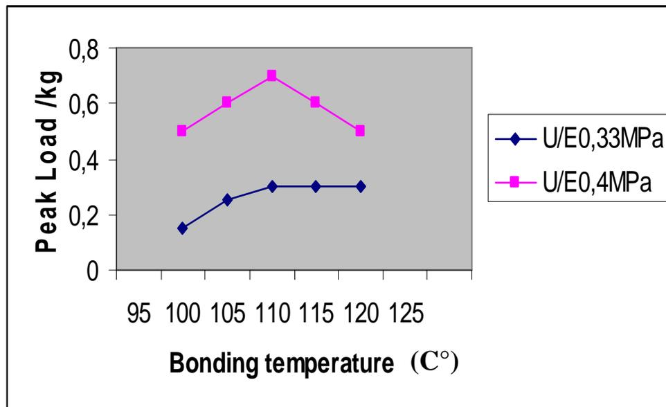
**Fig. (4): Relations between Bonding temperature and peak loads for 15/85 Usher/ ESTER**
