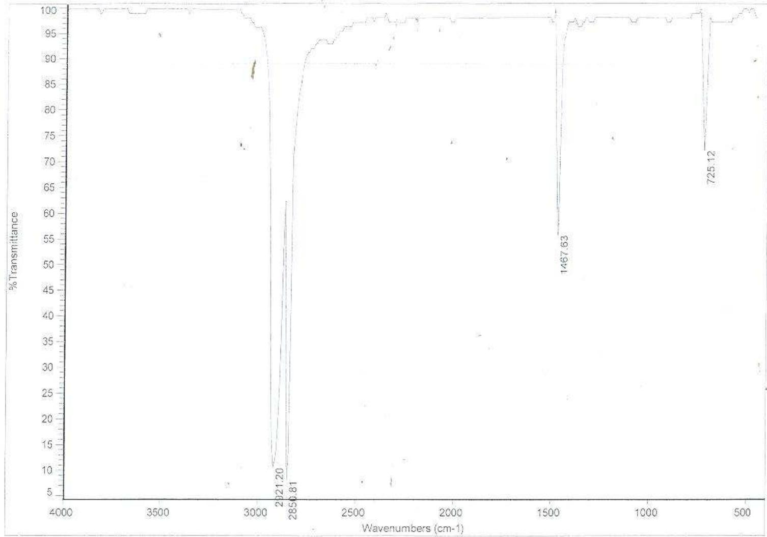
**Fig. (4): The results of the infrared spectrophotometry test of pure polyethylene reference sample**
