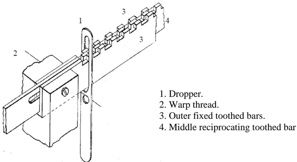
Fig 1.1 parts of the mechanical warp stop motion
