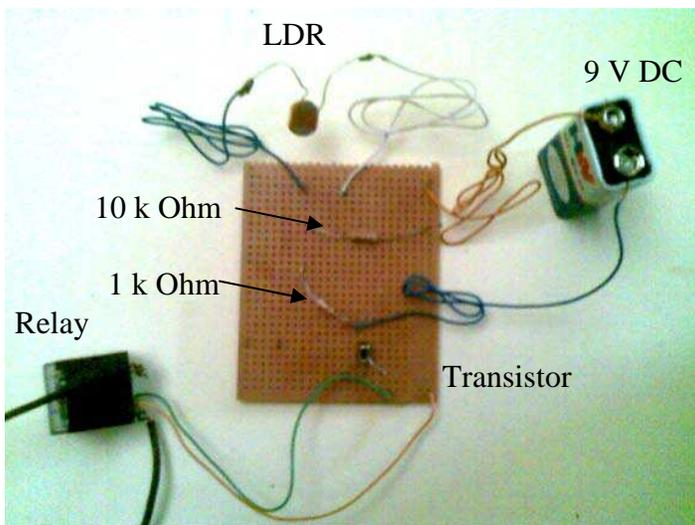
Picture 2.1: the electronic circuit connection
