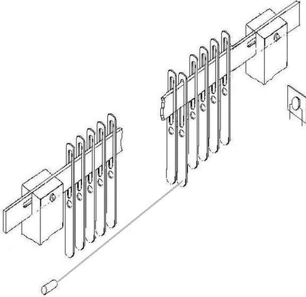
Fig (2.3): the falling of the dropper cutting the flow of the laser beam.
