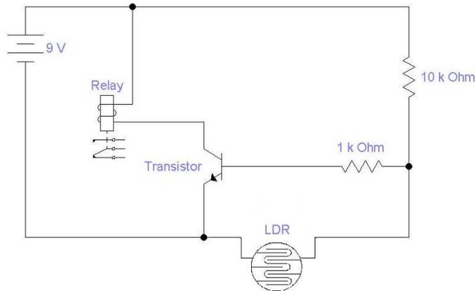
Fig 2.1: Connection of the electronic circuit components
