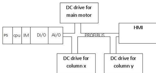
**Figure 1 Block Diagram of the New Control**
