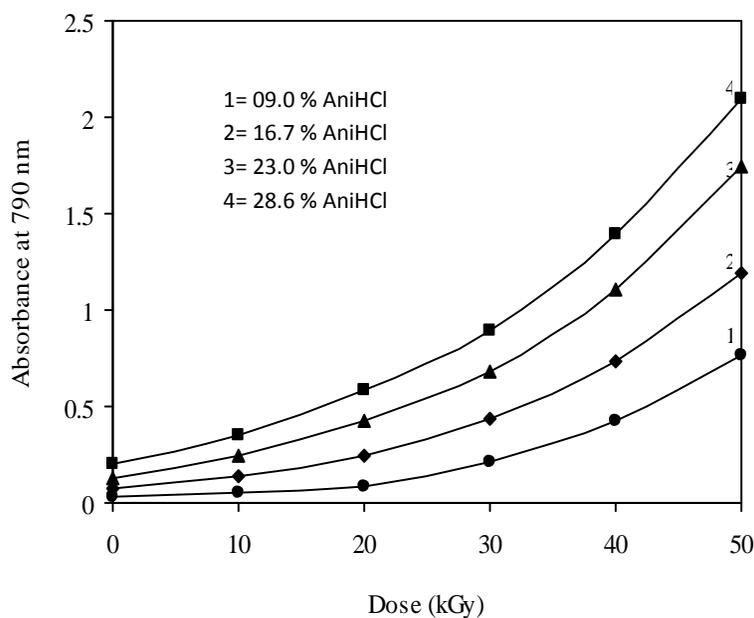
Fig. 3: Variations of absorbance band at 790 nm with radiation dose and the monomer concentration.
