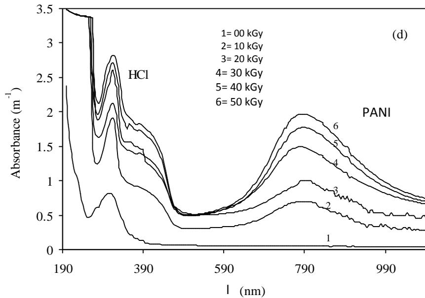
Fig 2: UV-visible spectra of PVA/AniHCl at different concentrations of AniHCl (a) 9.0, (b) 16.7, (c) 23.0 and (d) 28.6 % w/v and radiation dose up to 50 kGy.
