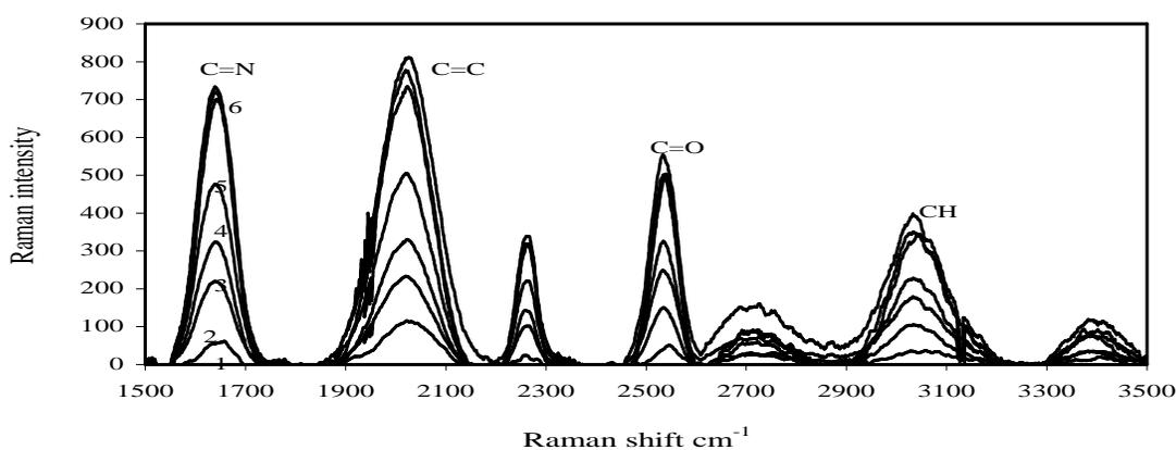
Fig 5: Raman intensity versus Raman shift spectrogram of the irradiated PVA/AniHCl up to 50 kGy.
