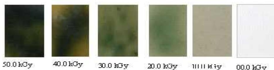
Fig. 1: the response of PVA/AniHCl composite to  $\gamma$ -irradiation, indicating the electrochromic and polymerization of aniline monomer.
