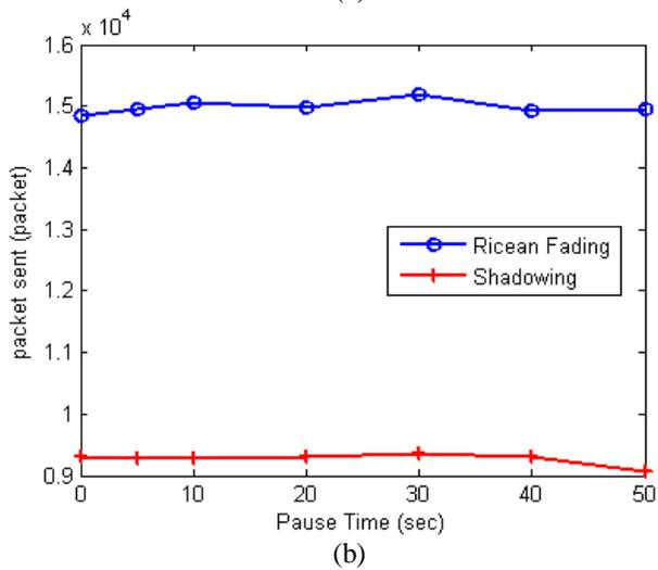
Fig. 4, packet sent Vs (a) Max Speed, (b) Pause Time
