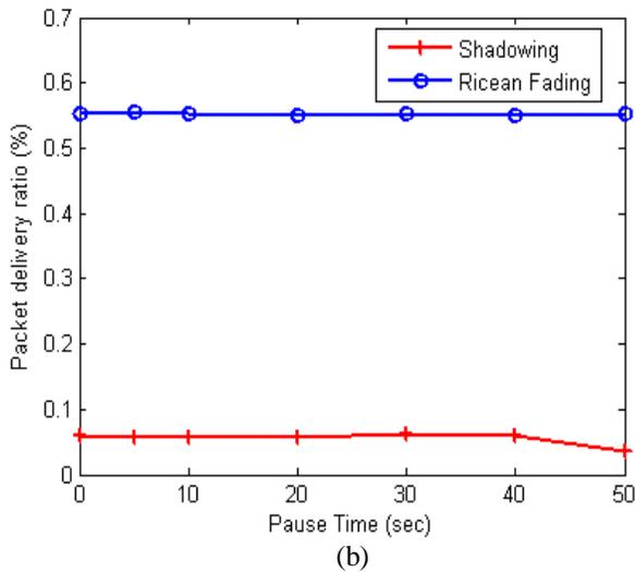
Fig. 7, Packet Delivery ratio Vs (a) Max Speed, (b) Pause Time
