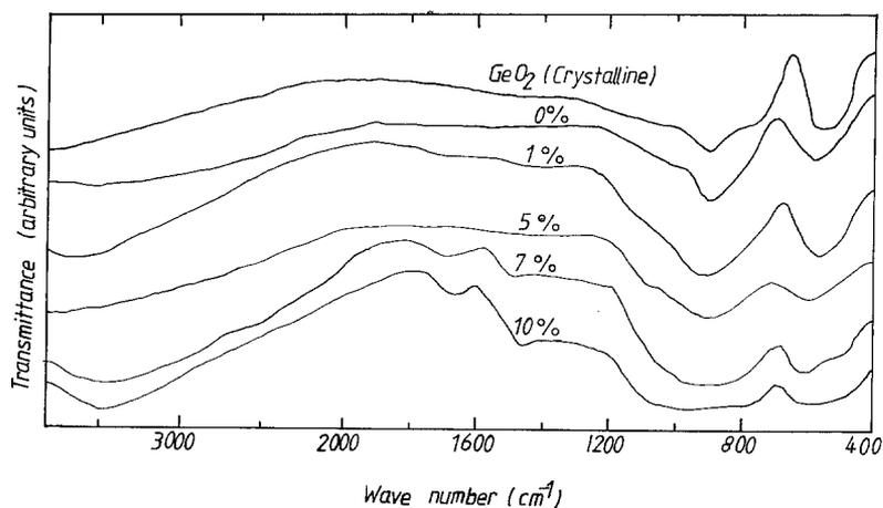
Figure 5 The infrared absorption spectra of five different samples (PrCl<sub>3</sub> content in mol% as indicated), and for crystalline GeO<sub>2</sub>.
