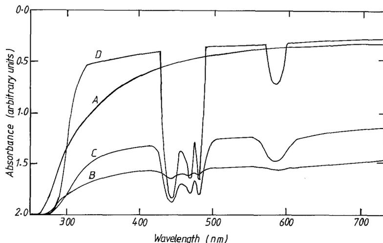
Figure 1 Absorption as a function of wavelength for glasses of different thicknesses and composition as given in Table I. Thickness: A, 1.02 mm; B, 1.2 mm; C, 1.73 mm; D, 2.00 mm.
