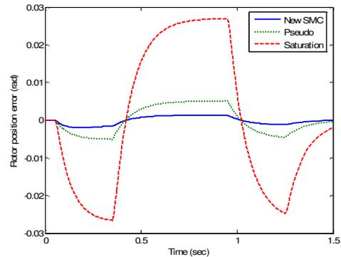
Fig. 3 Rotor position tracking error
