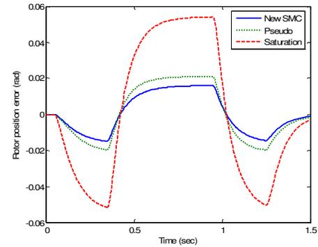
Fig. 9 Rotor position tracking error
