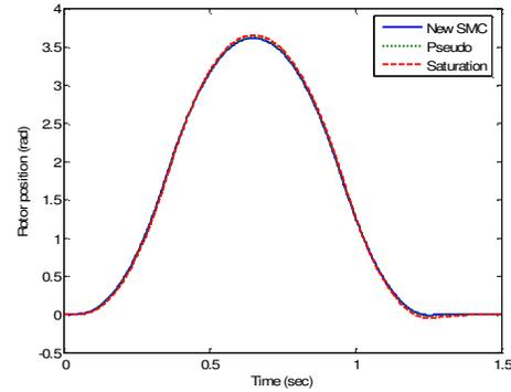
Fig. 8 Rotor position tracking performance
