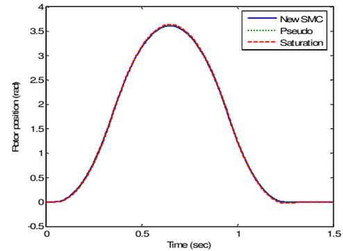
Fig. 2 Rotor position tracking performance
