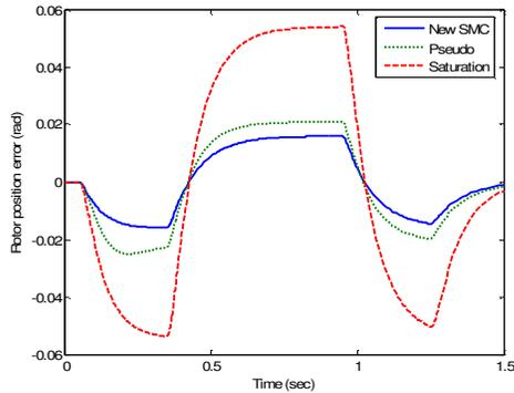
Fig. 6 Rotor position tracking error
