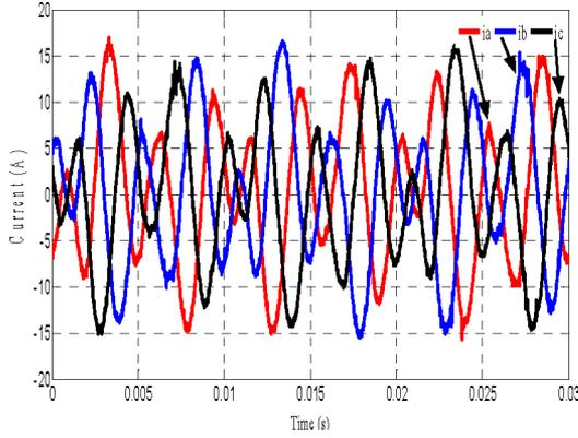
Fig. 3. Instantaneous phase currents with  $i_d = 0$  A during synthetic loading at full load and 100 Hz synthetic loading frequency.
