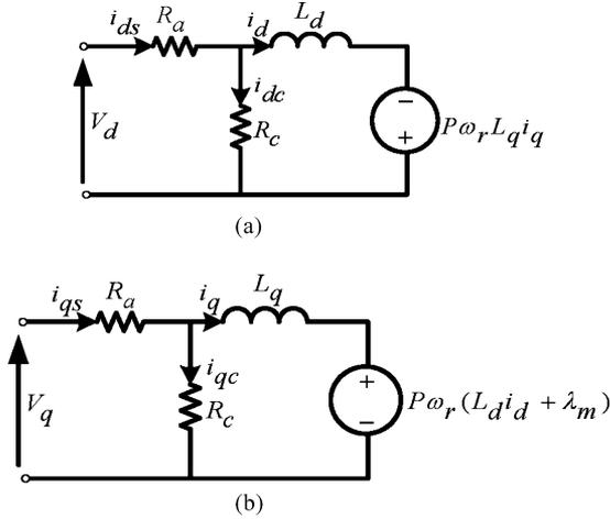
Fig. 1. (a)  $d$ - and (b)  $q$ -axis steady-state equivalent circuit of the PM synchronous machine.
