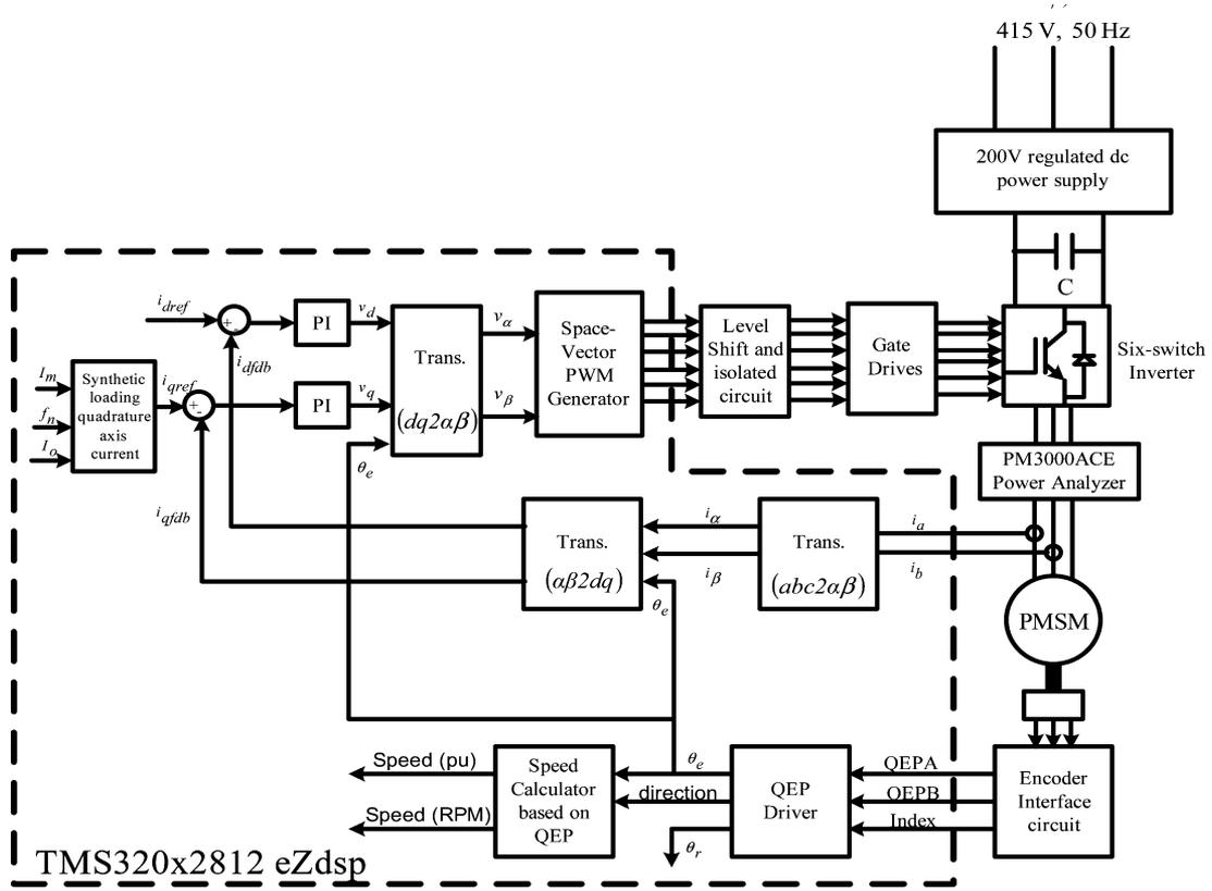
Fig. 2. Block diagram of vector control system for conducting the synthetic loading technique.
