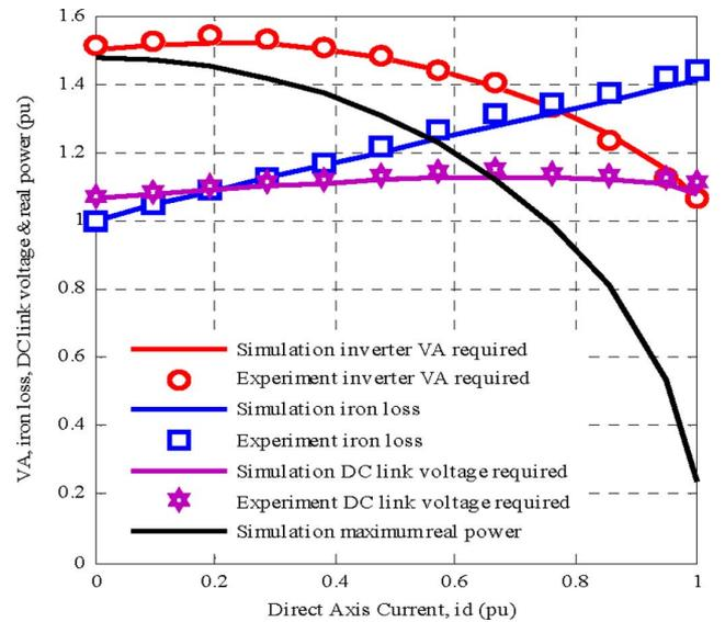
Fig. 5. Impact of direct axis current on the iron loss, inverter VA, inverter dc link voltage and inverter power.
