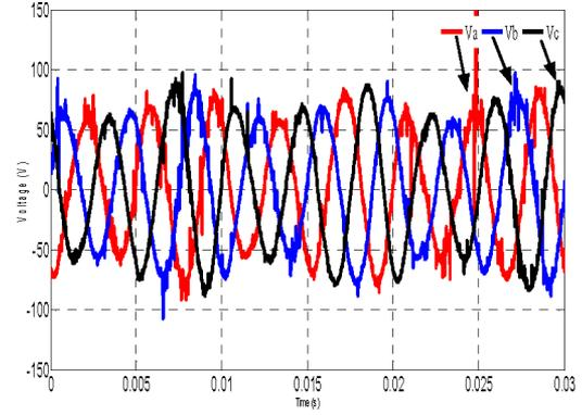
Fig. 4. Instantaneous phase voltage with  $i_d = 0$  A during synthetic loading at full load and 100 Hz synthetic loading frequency.
