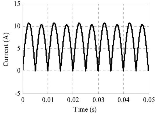
Fig. 7. Instantaneous rms line-current variation during synthetic loading at 100 Hz under full-load-torque condition.
