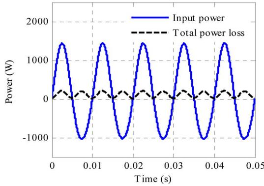
Fig. 3. Input power and total losses during synthetic loading for 100 Hz synthetic loading frequency.
