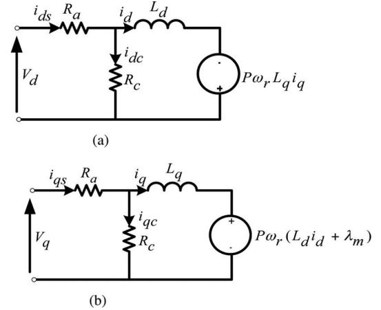
Fig. 1. (a)  $d$ - and (b)  $q$ -axis steady-state equivalent circuit of the PM synchronous machine.
