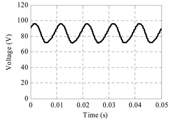
Fig. 5. RMS line-voltage variation during synthetic loading for 100 Hz under full-load-torque condition.
