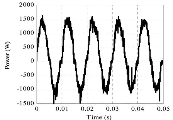
Fig. 13. Input power variation during synthetic loading for synthetic loading frequency 100 Hz.
