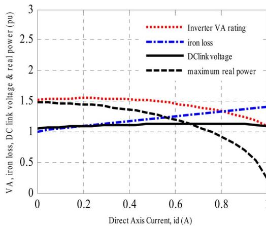
Fig. 8. Impact of direct-axis current on the synthetic loading performance.
