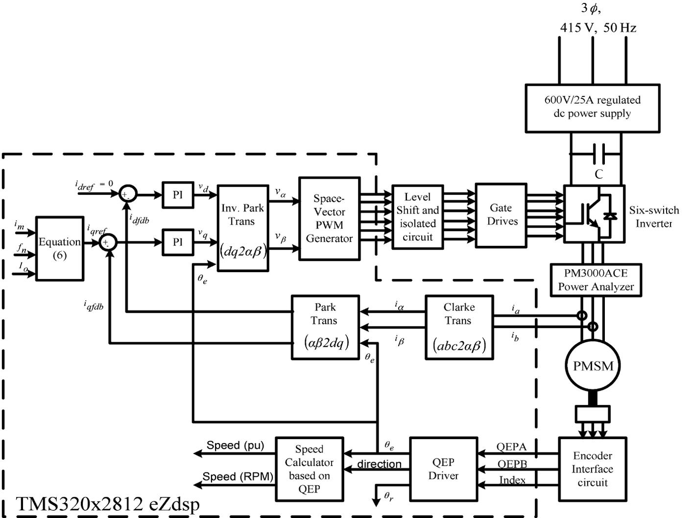
Fig. 9. Block diagram of vector control system for conducting synthetic loading technique.
