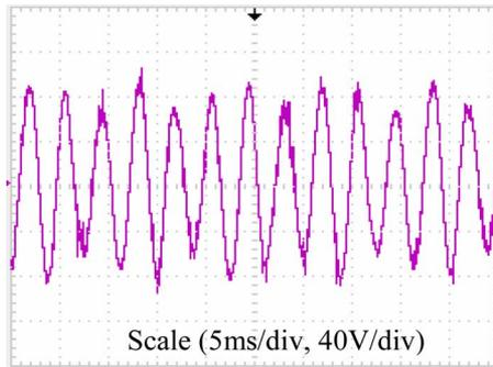
Fig. 10. Phase voltage during synthetic loading for synthetic loading frequency 100 Hz.
