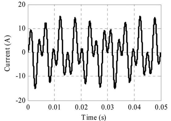
Fig. 6. Phase current during synthetic loading at 100 Hz.
