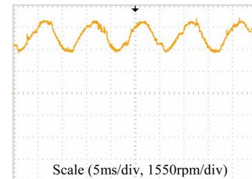
Fig. 12. Speed variation during synthetic loading for synthetic loading frequency 100 Hz.
