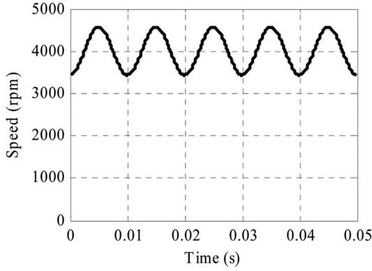
Fig. 2. Speed variation during synthetic loading for 100 Hz under full-load-torque condition.
