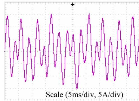
Fig. 11. Phase current during synthetic loading for synthetic loading frequency 100 Hz.
