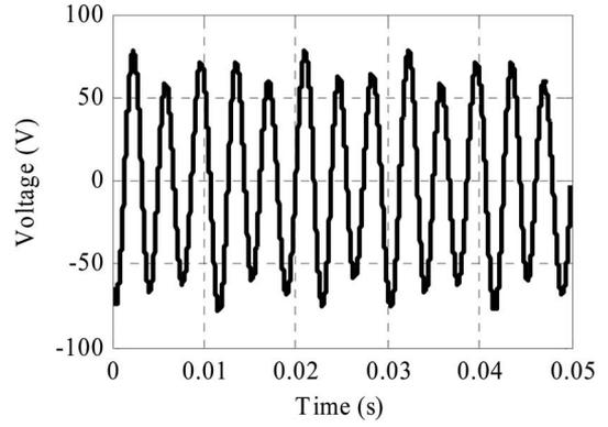
Fig. 4. Phase voltage during synthetic loading for 100 Hz synthetic loading frequency.
