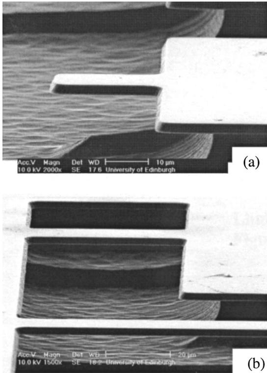
FIG. 3. SEM images of (a) a 25 μm long cantilever and (b) a 50 μm long bridge.
