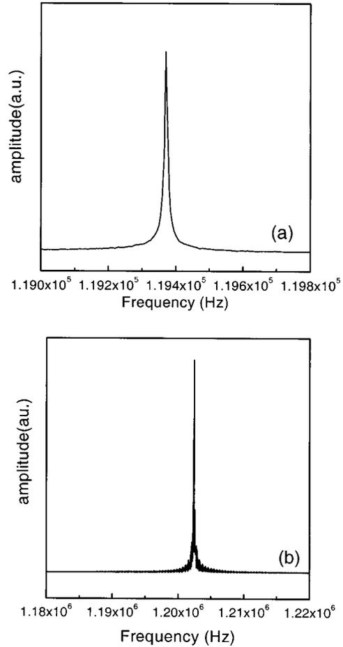
FIG. 4. Fundamental resonance peak of 200 μm long (a) cantilever (b) bridge structures.
