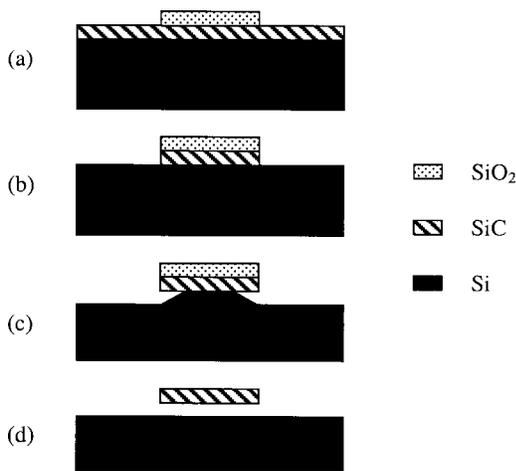
FIG. 1. (a)–(d) Schematic diagram of the processing steps to fabricate suspended SiC beams.
