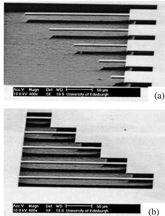
FIG. 2. SEM images of a group of free standing (a) cantilever beams with lengths of 25, 50, 100, 150, 200  $\mu\text{m}$ , respectively and (b) bridges with lengths of 50, 100, 150, 200, 250  $\mu\text{m}$ , respectively. All the beams are 15  $\mu\text{m}$  wide and nominally 2  $\mu\text{m}$  thick.
