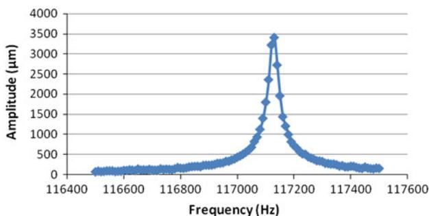
Fig. 2 The amplitude of resonance when applying 0.3 V ac and 0.2 V dc (before deterioration of the contact)
