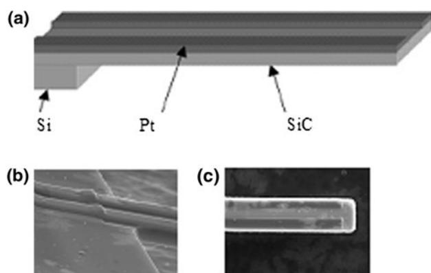
**Fig. 1** The designed excited cantilever with the platinum contacts **a**, **b** and **c** are the SEM images of the fabricated device
