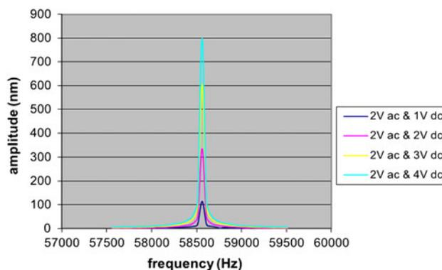
Fig. 4 The effect of dc bias at half resonance (58 kHz) as a result of rectifying contact
