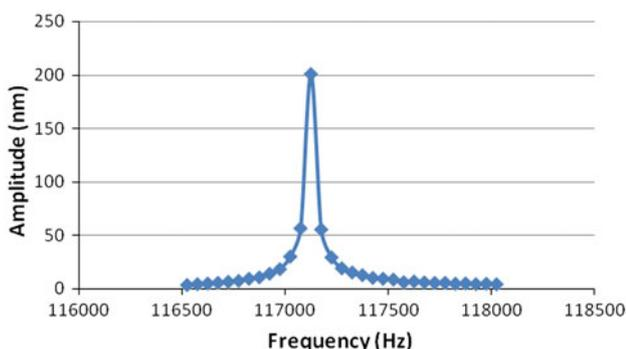
Fig. 3 The amplitude of resonance when applying 2 V ac and 1 V dc (after deterioration of the contact)
