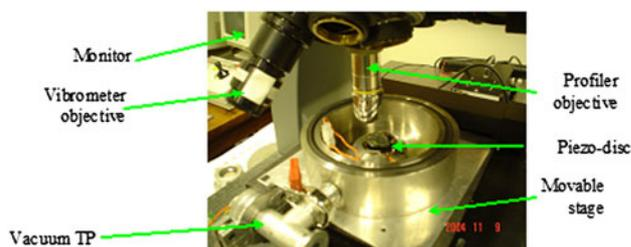
**Fig. 3** Testing equipment for actuation
