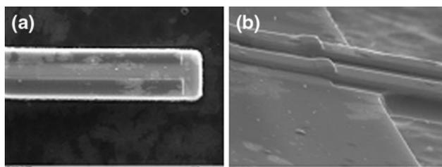
**Fig. 1** SEM images of the fabricated electrothermal SiC actuator; **a** is tip of the cantilever and **b** is the base of the cantilever
