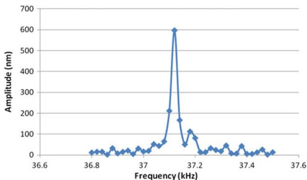
**Fig. 6** Signals addition: resonance detected when varying one signal (between 36.8 and 37.5 kHz) while keeping the other signal fixed at 80 kHz
