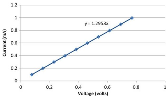
**Fig. 5** Voltage characterisation for SiC actuator ( $-DC$  current)
