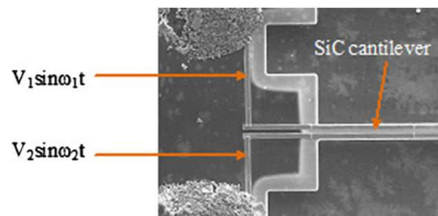
**Fig. 2** Applying signals on the cantilever
