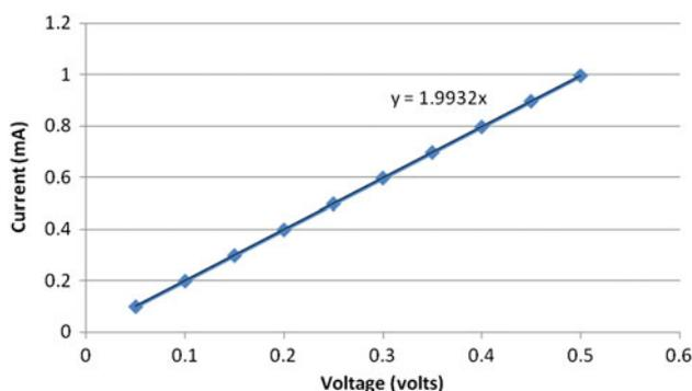
**Fig. 4** Voltage characterisation for SiC actuator (+DC current)
