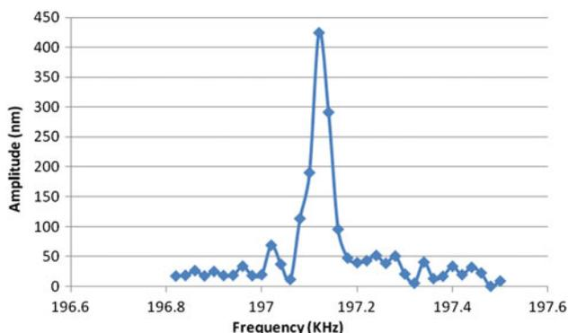
**Fig. 7** Signals subtraction: resonance detected when varying one signal (between 196.8 and 197.5 kHz) while keeping the other signal fixed at 80 kHz
