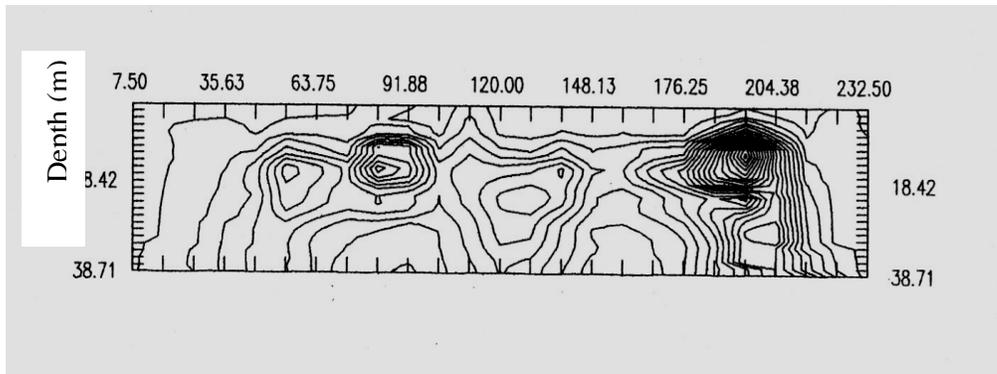
**Figure (4): Total Dissolved Solids Distribution along Line L-L<sub>1</sub> (Contours in**
