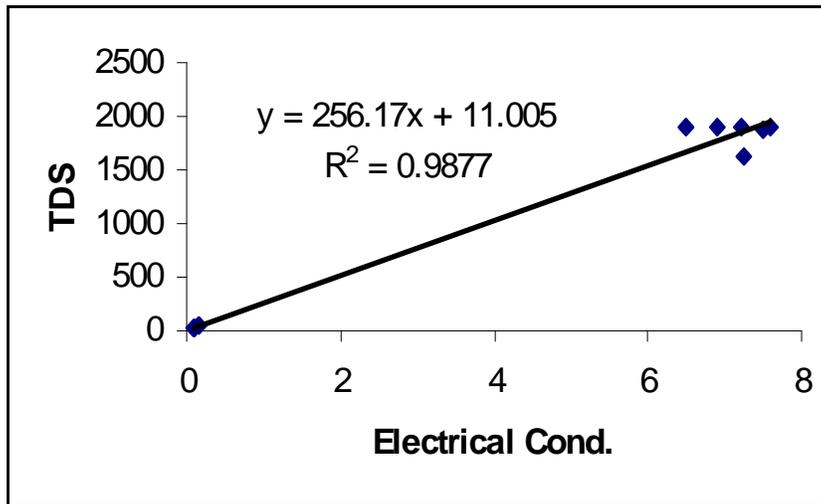
Figure (2): Relationship between Total Dissolved Solids (TDS) and Electrical Conductivity (EC)
