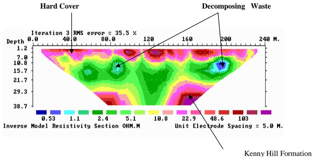
Figure (3): Resistivity Image along Line L-L<sub>1</sub>
