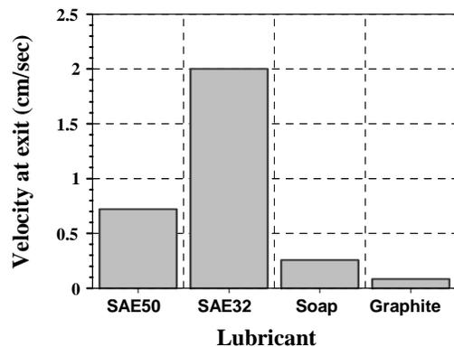
Fig. (3) Effect of Lubricant on Extrusion Velocity
