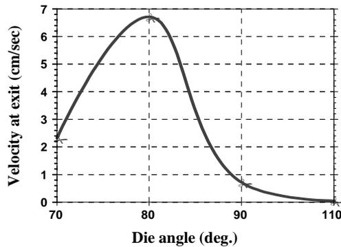
Fig. (2): Effect of Die Angle on the Exit Velocity
