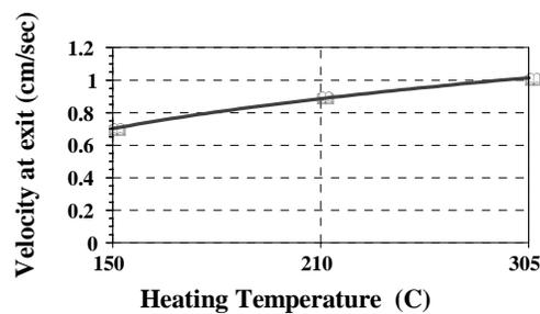
Figure (1) Effect of temperature on extrusion velocity
